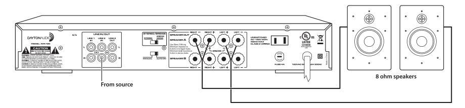
**Bridged Mono Connection Diagram**
